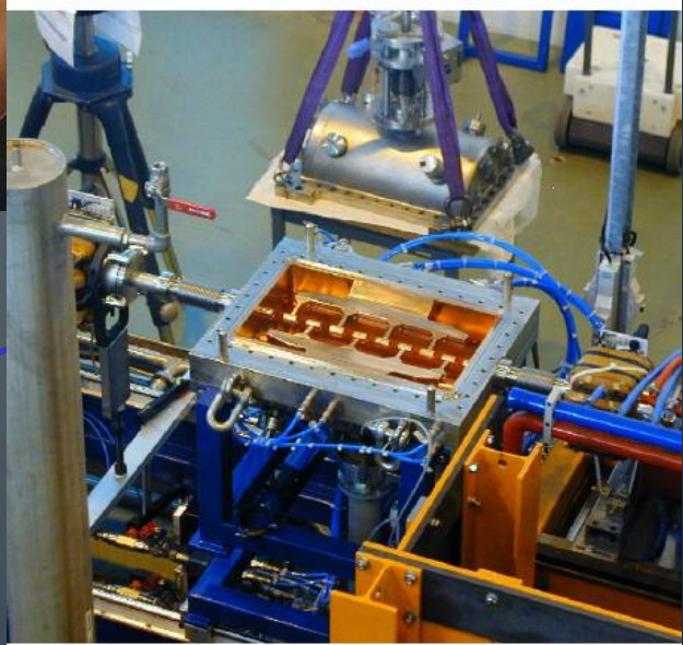
Rex-Isolde IH (CERN), 202.6 MHz
