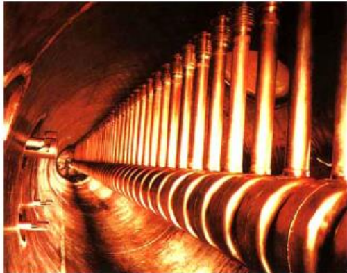
Saturne DTL (Saclay) : -> 20 MeV, 200 MHz
